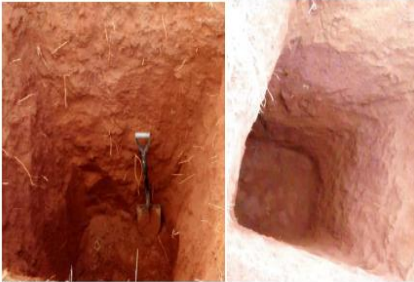
Figure 5-1(c)–Selected trial Pit (TP02 & TP03) photos at the proposed Lilambo industrial Area.
